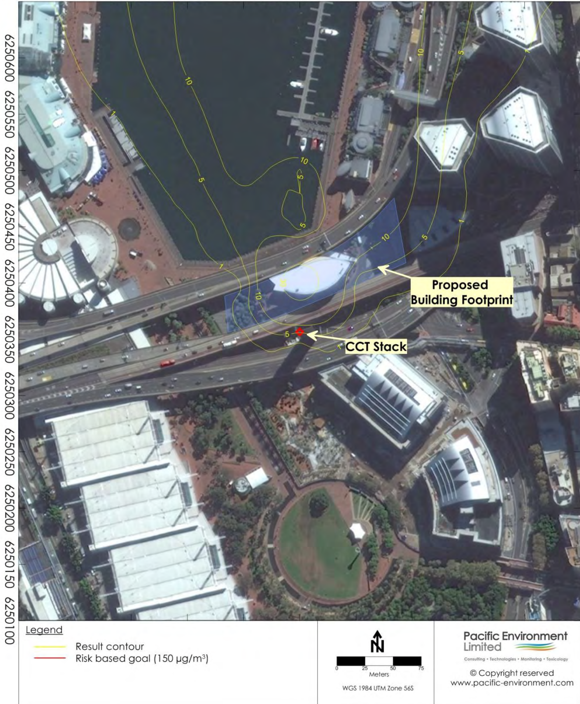
60 m – Peak Emissions Scenario – 1-Hour \text{NO}_2 Concentration (Goal – 150 \mu\text{g}/\text{m}^3 )
