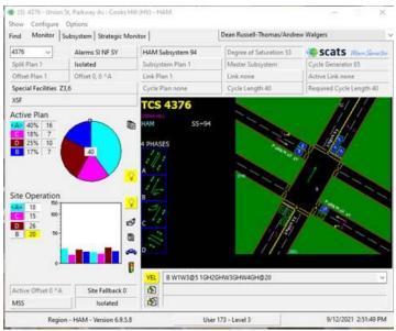
• Intergreen (yellow/red times) need to be updated to be as per SCATS time settings. All red times for all phases are 4 seconds here due to the large clearance of the median
