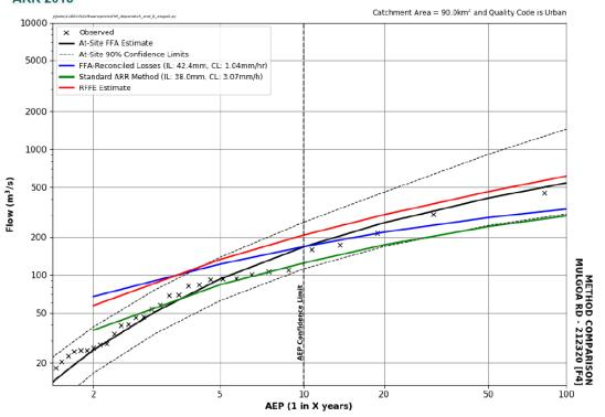
Figure 4-13 Comparison of flow estimation methods at Mulgoa Rd Gauge (WMA Water, 2019)
