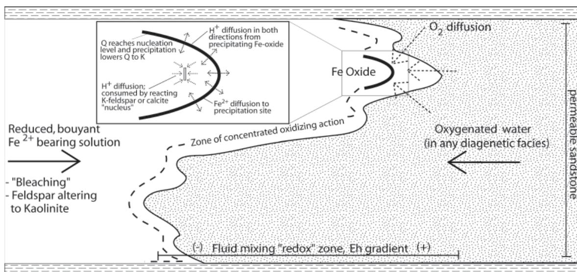
**Figure 4** Generalized conceptual model of an oxidation-reduction front with precipitation of ferric oxide near the interface between oxidizing, O<sub>2</sub>-bearing water and reduced, Fe<sup>2+</sup>-bearing waters. A reduced, Fe<sup>2+</sup>-bearing solution moves to the right into a region of porous rock containing oxygenated water. (From Beitler et al. 2005, Fig. 12)
