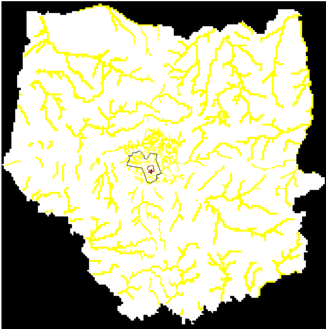
Figure 11 Groundwater Model Boundary Conditions – Drain (DRN) Cells
