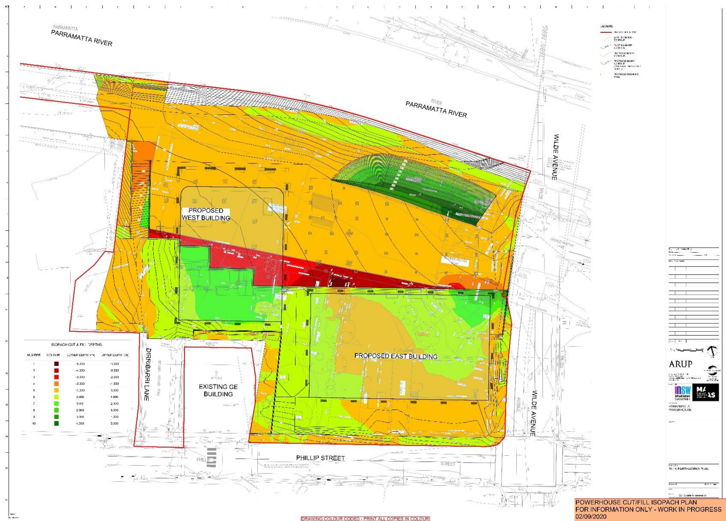
Figure 2-1 Plan of proposed cut and fill across the study area. Note the dark red excavation for the undercroft. (Source: ARUP)
