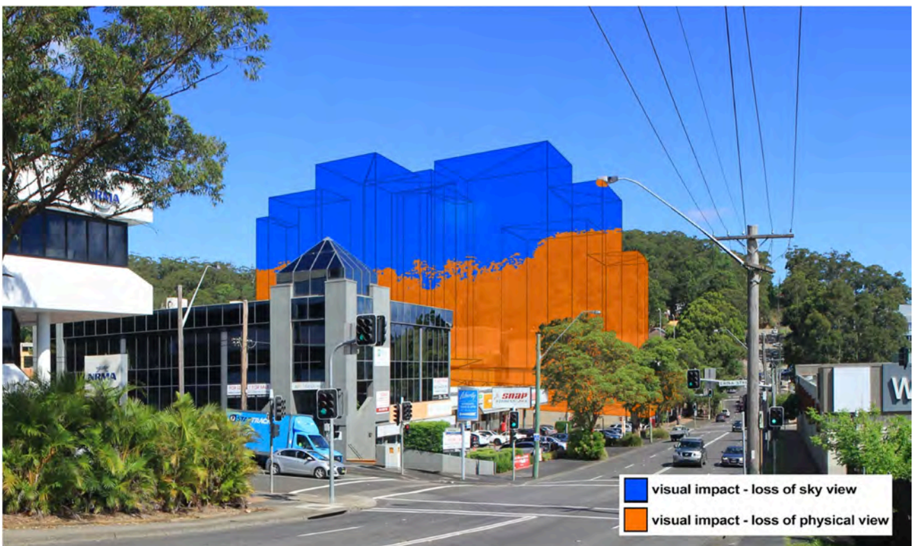
Figure 9: Example of assessment of visual impact ratios - sky and physical content view loss.
