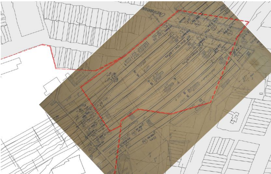
Figure 26: 1948 - Plan showing track layout, extant structures including the ventilation shafts from the engine dive that passes directly under Platform 1. Source: Drawing courtesy of Estate of Martin Davies from private report titled NSWGR - Devonshire St to Illawarra Junction Part 1 - University Historical Archaeology II Project 1978 contained in Paul Davies, p.11 with TZG overlays of 2018 LEP and site boundaries of Redfern Station and Eveleigh Railway Workshops.
