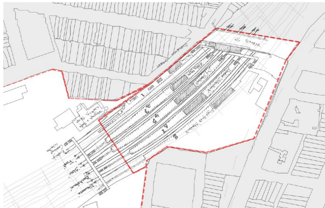
Figure 22: 1915 - The layout of the station at the completion of the 1912-15 works with two double faced standard island buildings and a single faced standard island building on platform 8. Note the footbridge at the southern end of the station, beyond the end of the platforms.
