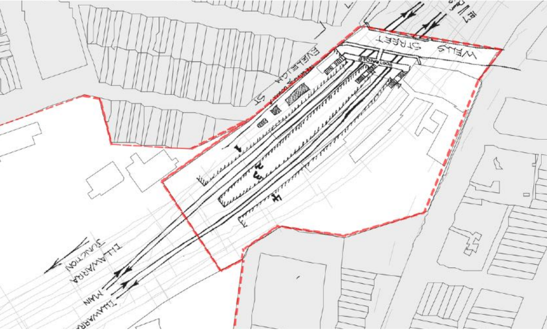
Figure 20: 1883 - The 1883 layout or the as-built layout of the station two side platforms and an island platform but only buildings on the No 1 platform. Wells Street Bridge was completed in 1884 with a simple stair access to the platforms. Source: Drawing courtesy of Estate of Martin Davies from private report titled NSWGR - Devonshire St to Illawarra Junction Part 1 - University Historical Archaeology II Project 1978 contained in Paul Davies, p.6. with TZG overlays of 2018 LEP and site boundaries of Redfern Station and Eveleigh Railway Workshops.
