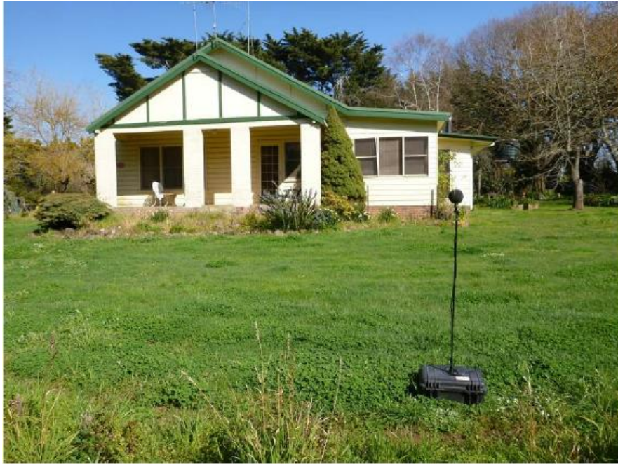
Figure 5.3 Photo of noise logging equipment installed at House HN05.
