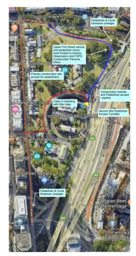
Figure 4 Construction works and Pedestrian interfaces
