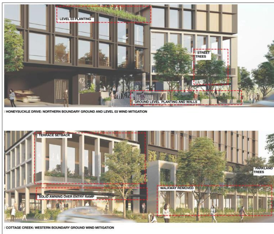
Figure 9 – Concept Wind Mitigation Measures
