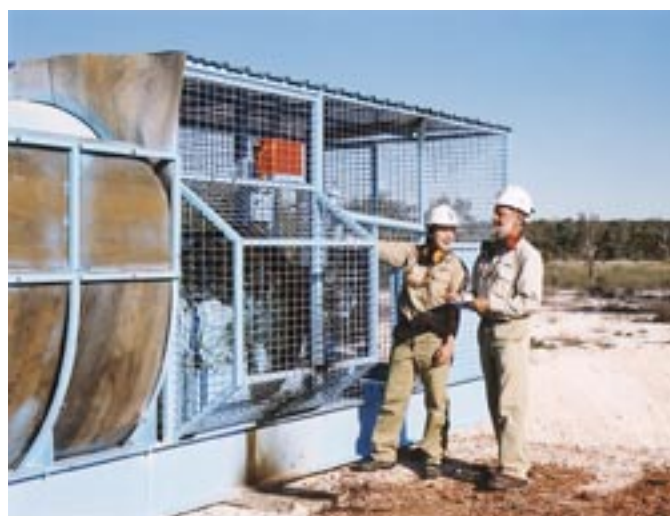
Renae Coleman and Warwick Schofield, Mine Safety Officer and Environment Officers at Lightning Ridge, assessing mechanical safety standards, maintenance and guarding on an agitator used to wash opals from mullock dug from opal mining
