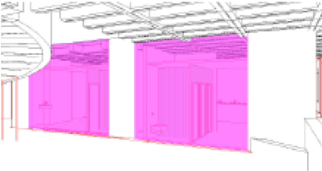
Figure 3: section of concrete wall to be removed (Source: Lacoste Stevenson)
