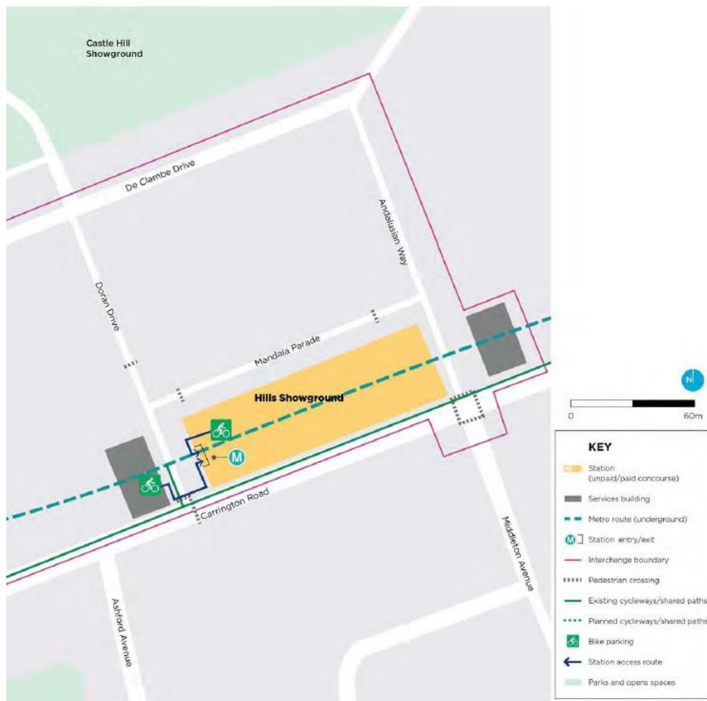
Figure 3–7 Cycling facilities and access between bike parking and station entry at Hills Showground Station
