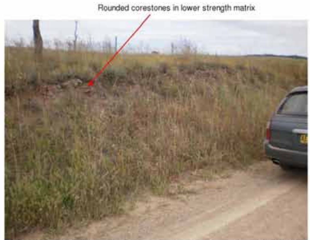
Photo 9: 2m cutting in basalt in Lookout Road near the intersection with Ophir Road.
