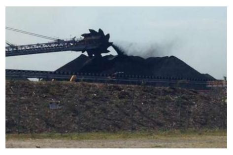
Figure 2. Kooragang coal loader operating in a dry westerly wind
