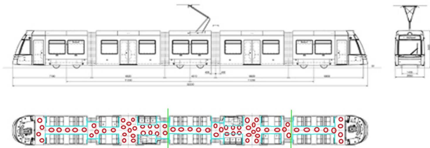
■ seated passenger, ○ standing passenger at operational capacity
