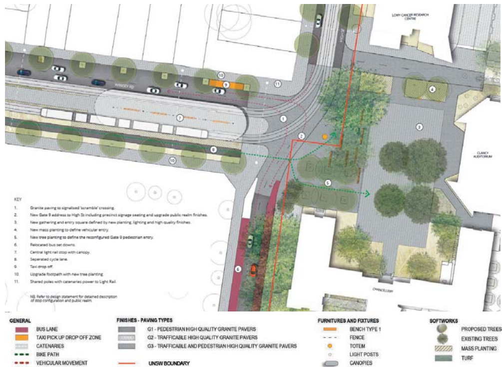
Figure 25 – UNSW High Street Stop - Landscape and Groundplane Plan
