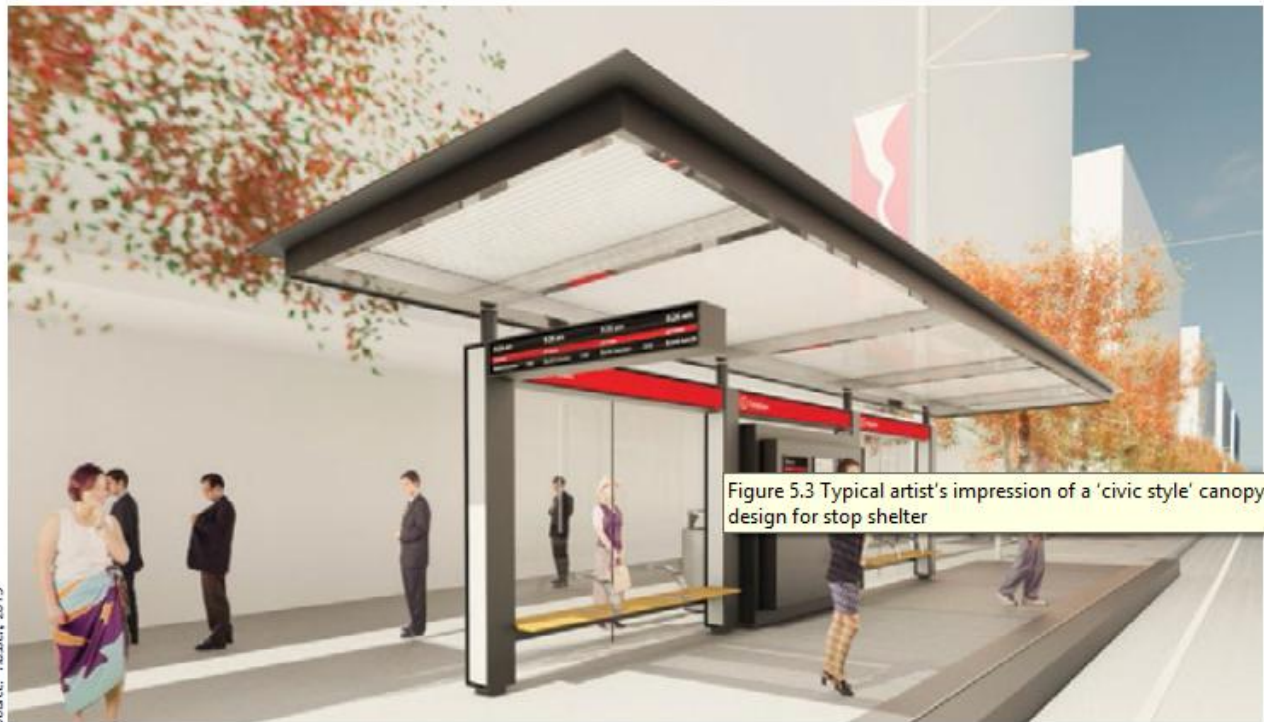
Figure 5.3 Typical artist's impression of a 'civic style' canopy design for stop shelter
