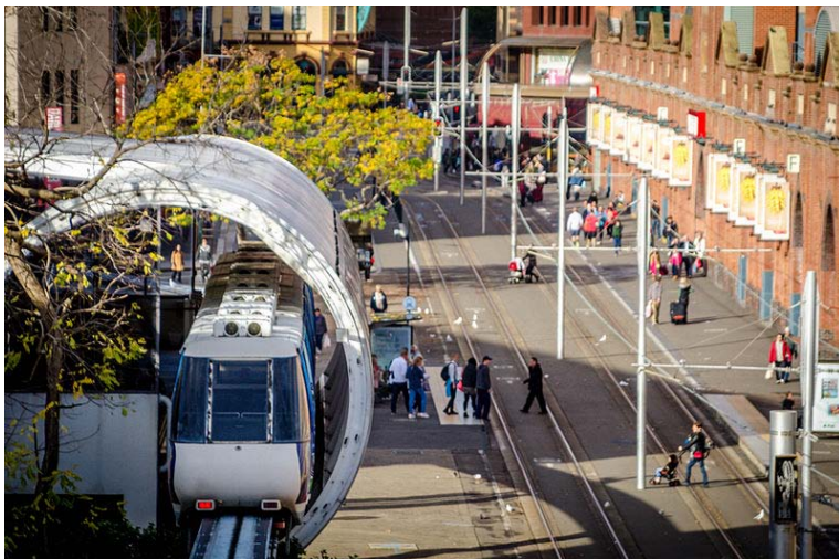
Figure 2. Safe and unsafe practice in light rail: The safety principles of reserved track and separation of passengers from the rail corridor and road traffic are evident in the Sydney monorail stop (left ) but absent in the inner west light rail stop where uncontrolled track crossings occur (right) (photograph from Wikipedia).
