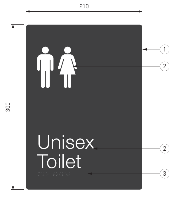
01 FRONT ELEVATION IN04.1-UNISEX TOILET ENS/WC-B/WC-PU SCALE 1:4
