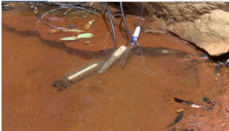
Picture 3: Severe longwall induced subsidence fracturing of Redbank Creek, near Picton. This was the site of a ground water 'vent' where upwelling groundwater flowing into Redbank Creek, through a fresh subsidence fracture. Water quality very extremely poor for the aquatic ecosystem with very low dissolved
