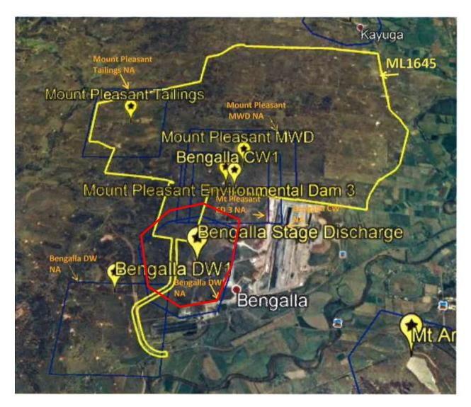
In Figure above the yellow polygon delineates Mount Pleasant Mining Lease ML1645. Blue polygons delineate Notification Areas around Prescribed dams. The red polygon is the Notification Area around what was Bengalla Staged Discharge Dam (BSDD). The BSDD no longer exists having recently been mined through by Bengalla Mine.
