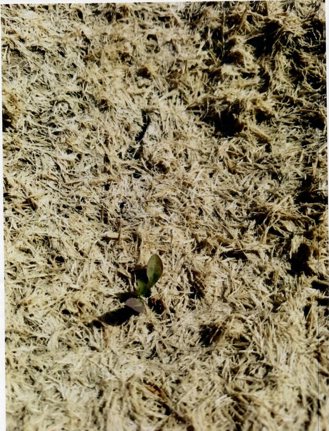
Figure 2. Hydromulch trial 26/09/19. Germination success for rye grass blend. Note the fibre is intact and forming a consistent cover.
