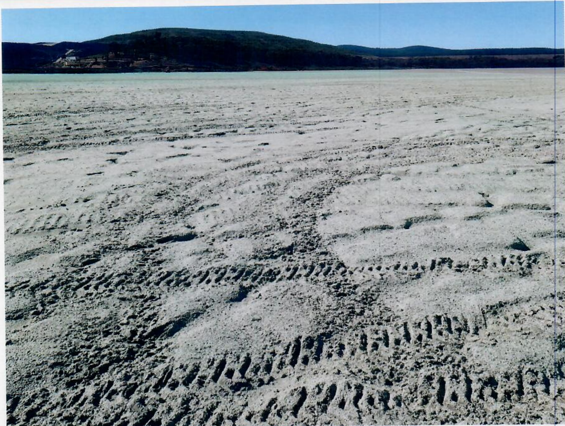
Figure 3. Hydromulch trial 16/08/19. The Hydromulch falls into the holes left behind from the Panther tracks.
