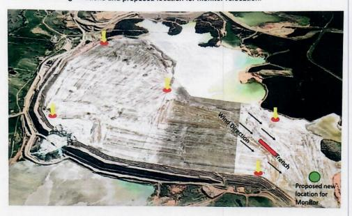
Trench identified as the root cause for the dust lift-off - before and after treatment.
