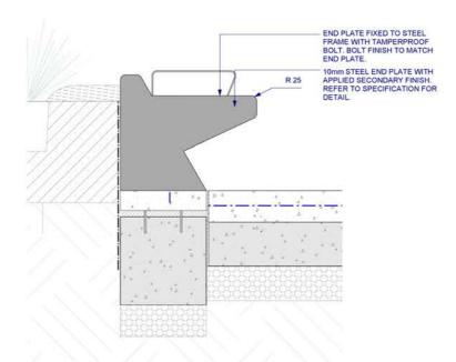
WALL TYPE 1 - PRECAST CONCRETE WALL WITH INTEGRATED TIMBER BENCH TYPICAL ELEVATION
