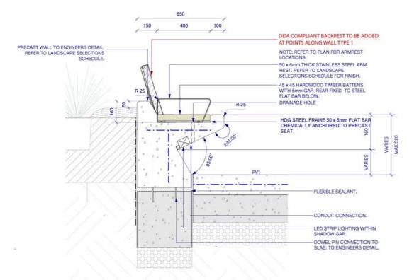
WALL TYPE 1 - PRECAST CONCRETE WALL WITH INTEGRATED TIMBER BENCH TYPICAL SECTION
