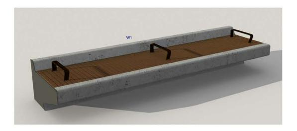
WALL TYPE 1 - PRECAST CONCRETE WALL WITH INTEGRATED TIMBER BENCH
