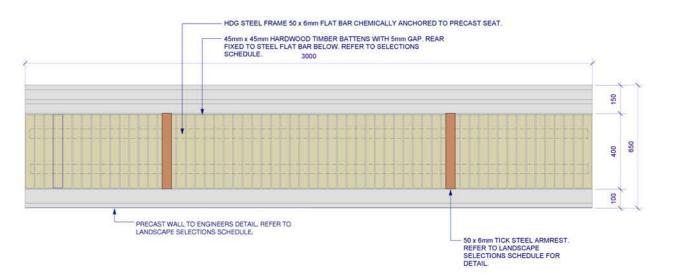
WALL TYPE 1 - PRECAST CONCRETE WALL WITH INTEGRATED TIMBER BENCH
