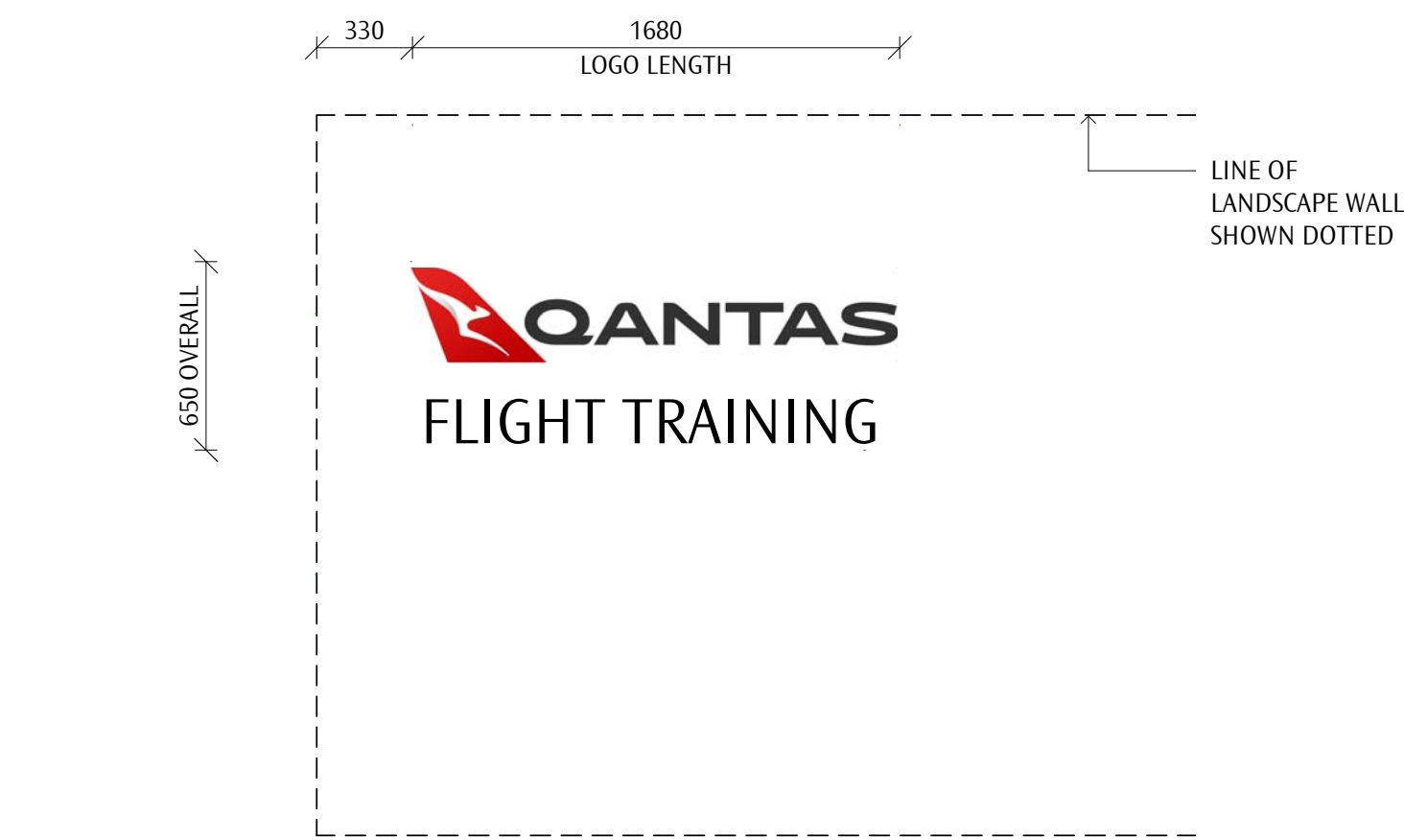
01 DETAIL ELEVATION - F-SN-QF/01 - NORTH ROAD 1 : 25
