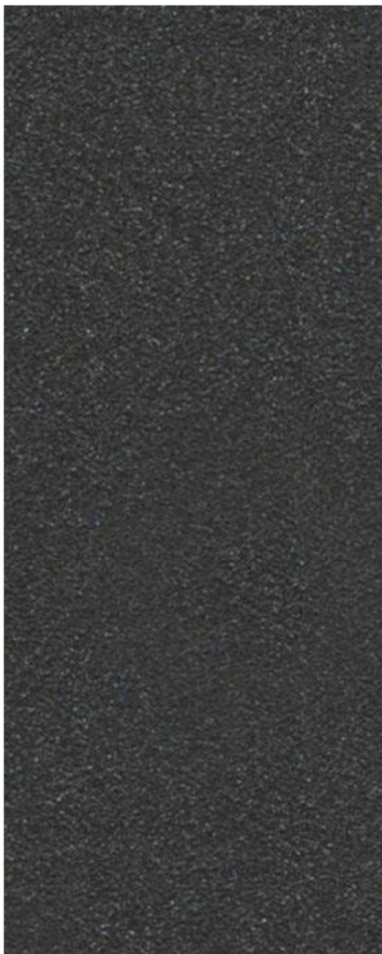
5. BALUSTRADE/ SCREEN - PAINTED STEEL; PAINT FINISH - DARK GREY MICACEOUS OXIDE
