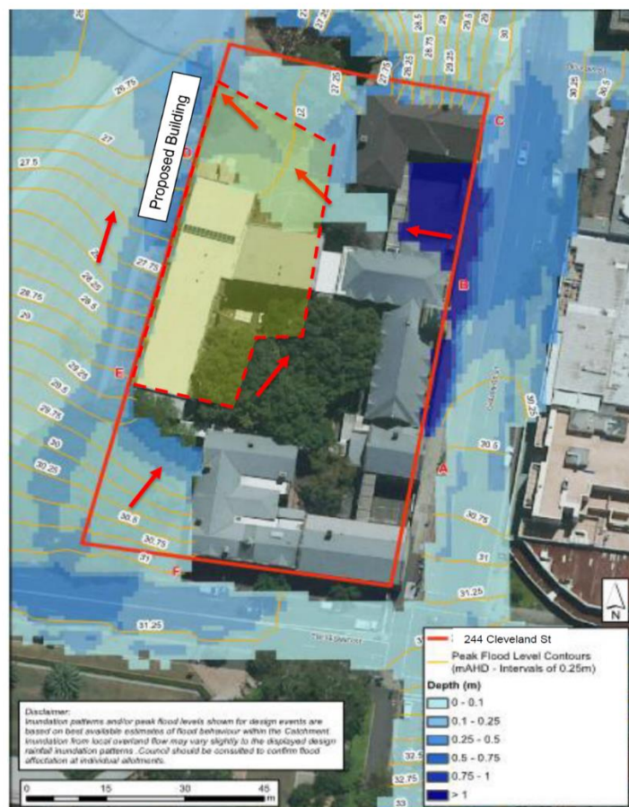
Figure 2 –Flood depth and level contours for 1% AEP flooding event
