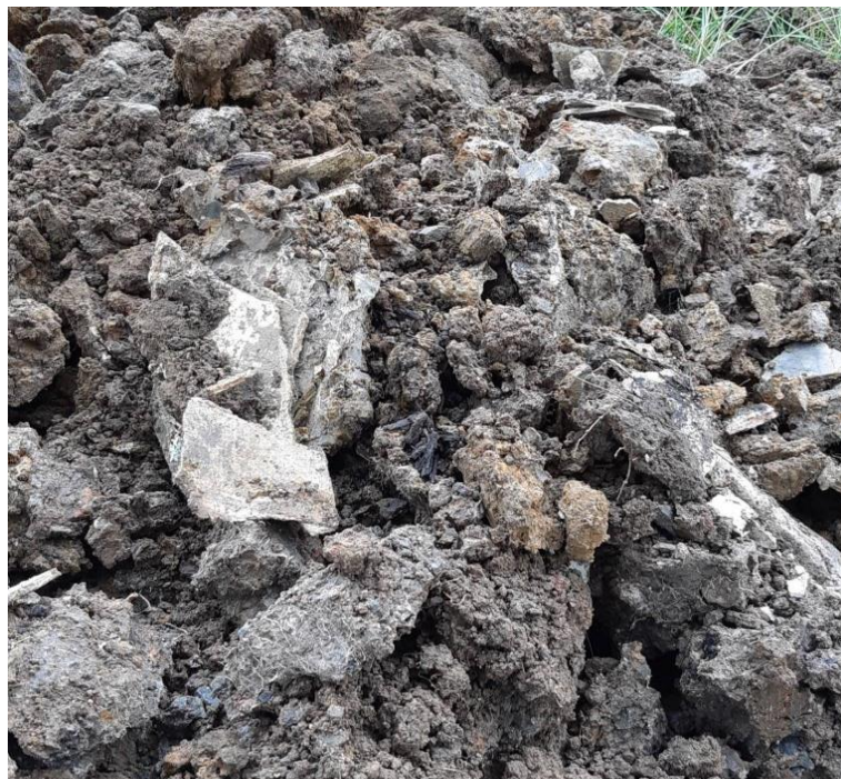
Photo 8 - ACM impacted fill excavated from test pit 205
