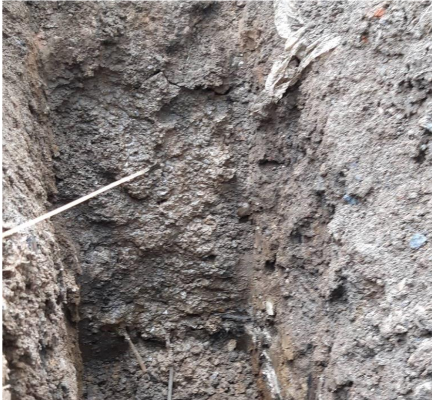
Photo 7 - Test pit 205 where ACM was identified in fill
