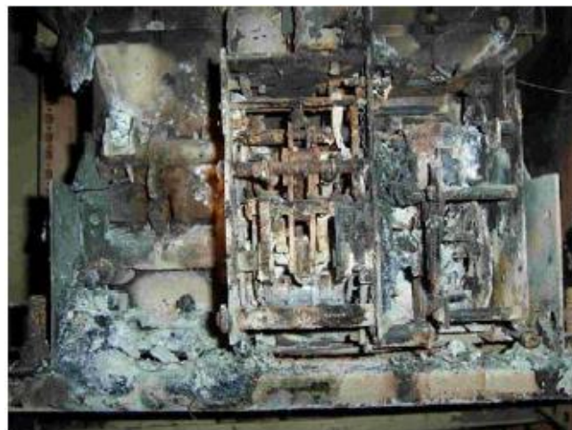
Figure 3. Power of a 1MW wind turbine-destroyed by fire (source Allianz)
