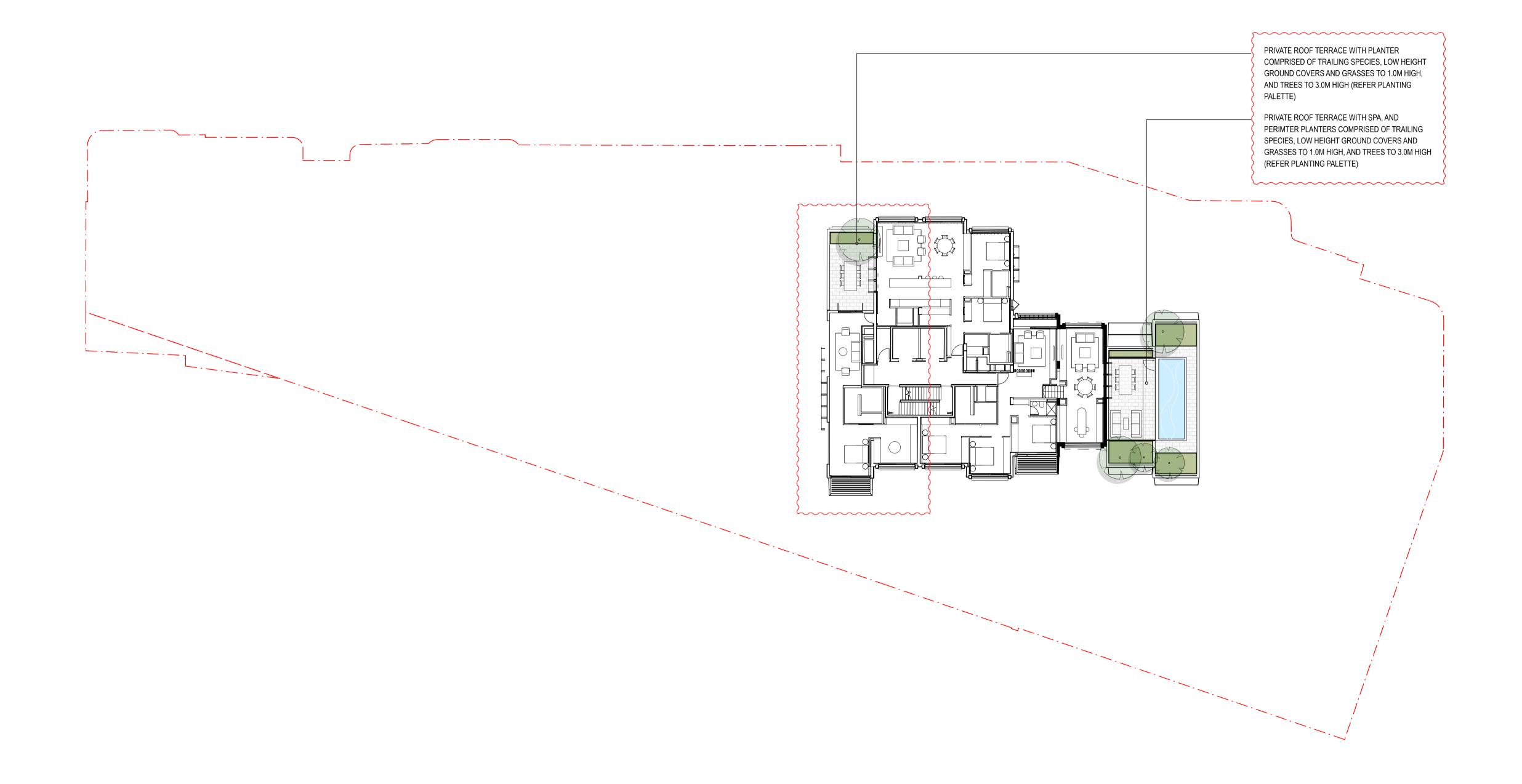
Roof Garden maintenance via sequence of static line connections and fixed ladders and manholes. Refer to maintenance access diagram for method and sequence of access to each roof
