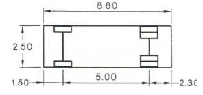
Height: 3.8m Turning Radius: 10.0m Overall Length: 8.8m Overall width: 2.5m
