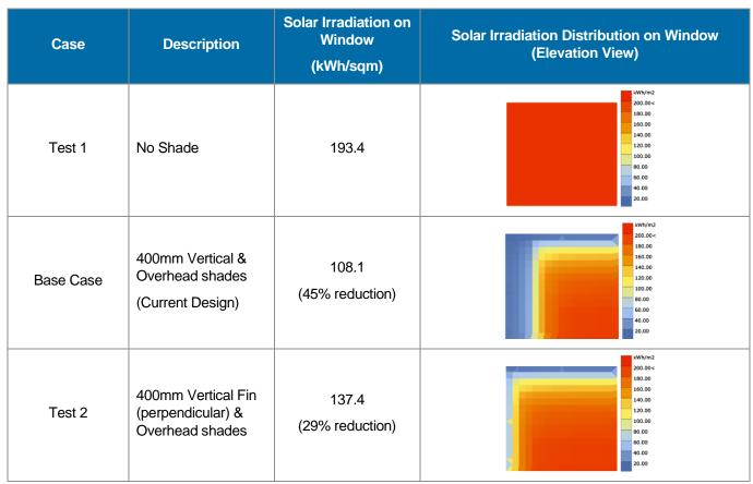
Table 1 Simulation Results – Solar Irradiation Distribution on Window for Study Period 1 Dec – 28 Feb
