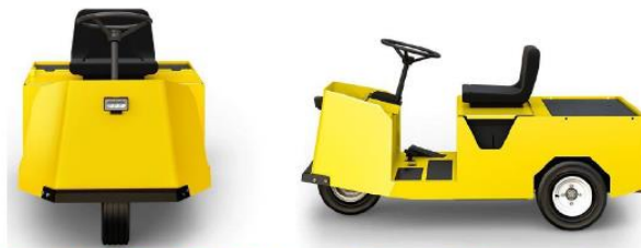
Figure 10: Typical Electric Ride On Tug Device used by the caretaker for the movement of 660L & 1100L bins within the development
