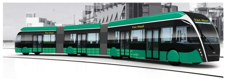
15 CNG-fueled, 78-foot ExquiCity 24 hybrid buses by Belgiumâs Van Hool for BRT service in Malmo, Sweden will have new Euro6 MAN engines, series hybrid electric drivelines by Siemens, and Type III carbon fiber-on-aluminum fuel cylinders by Luxfer-Dynetek.
