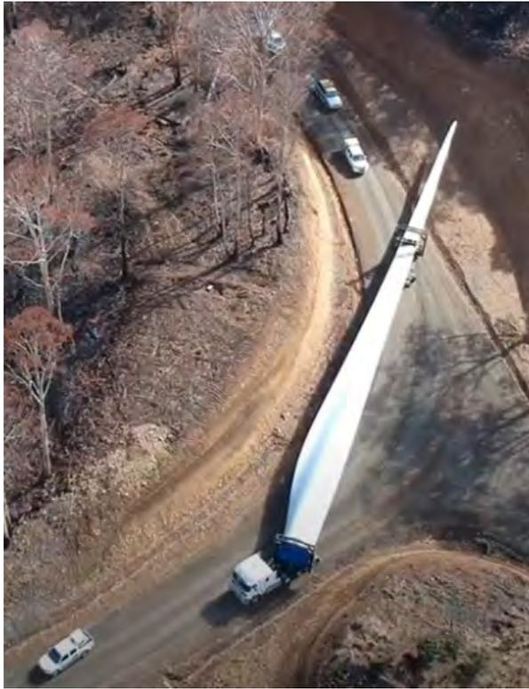
3. Transporting the turbine elements requires substantial access tracks given the length of the components being transported (photo source: Goldwind. Cattle Hill Wind Farm, Tasmania).
