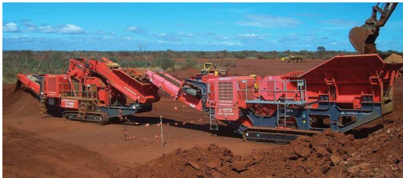
Figure 2-9 Example of a mobile crushing and screening plant process as proposed for use within the earthwork material sites
