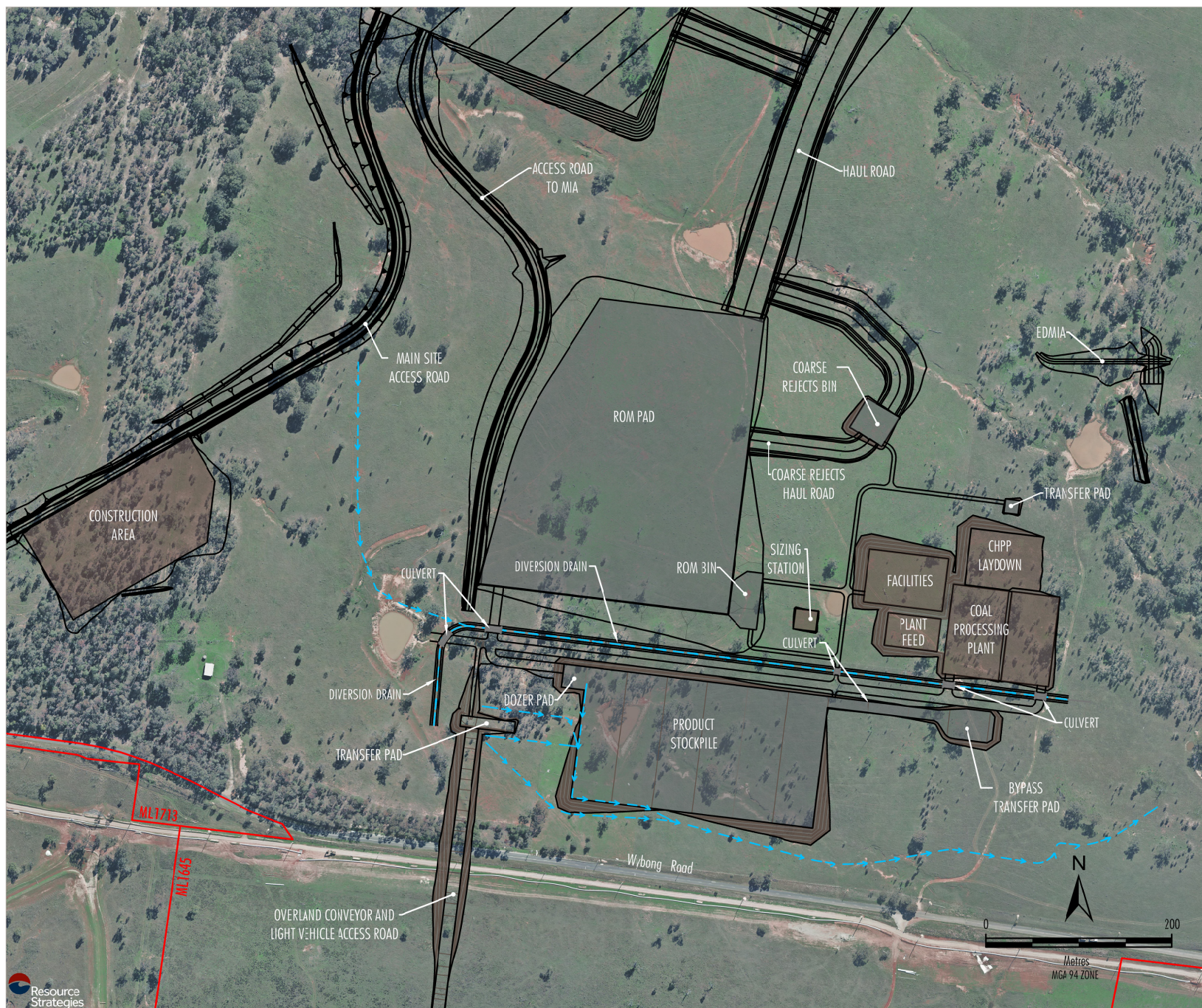
MACHEnergy MOUNT PLEASANT OPERATION Provisional General Arrangement of the CHPP and Materials Handling Area
