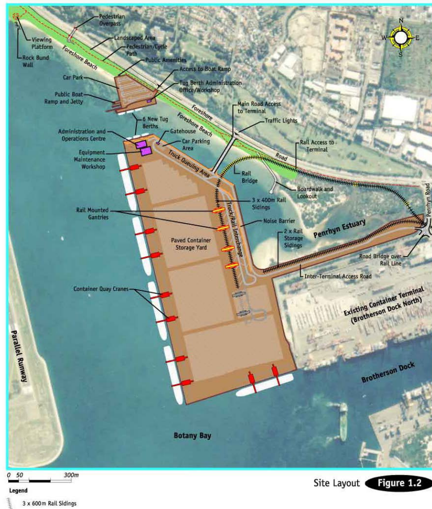
Figure 2-1: Extract of EIS ‘Site Layout’ showing the general approved site layout and buildings arrangement.
