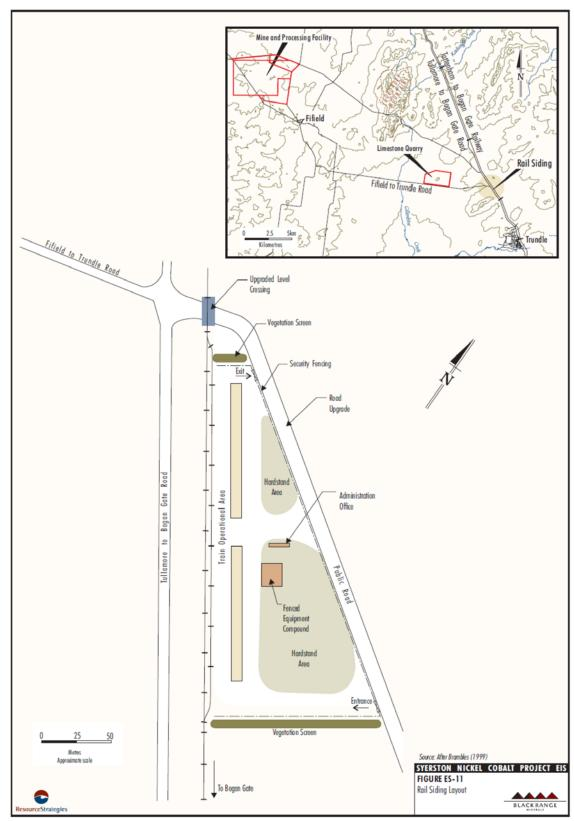
Figure 8: Rail Siding Layout
