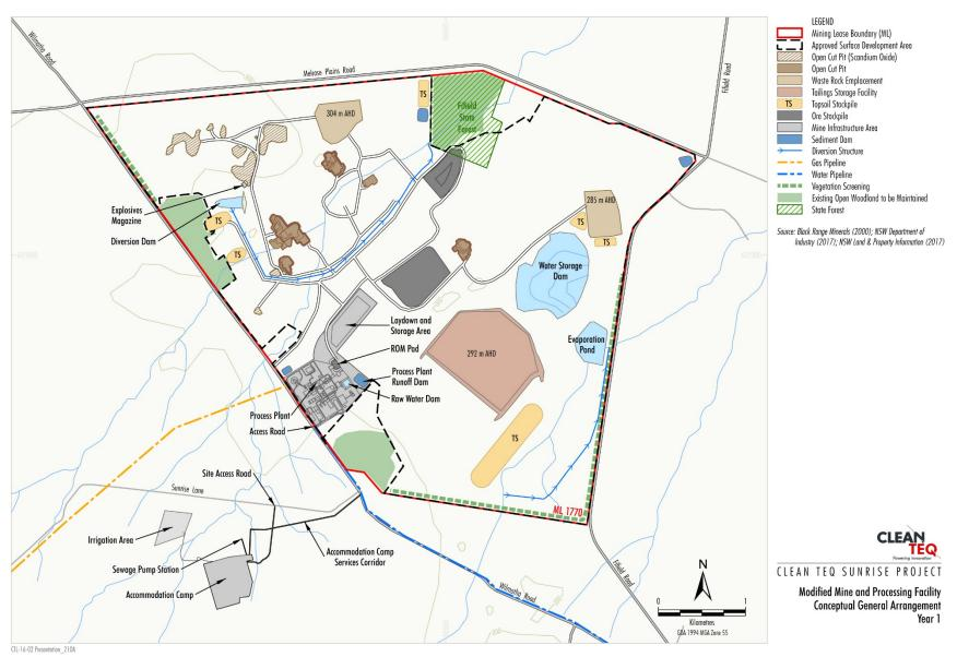
Figure 3: Mine and Processing Facility – Year 1
