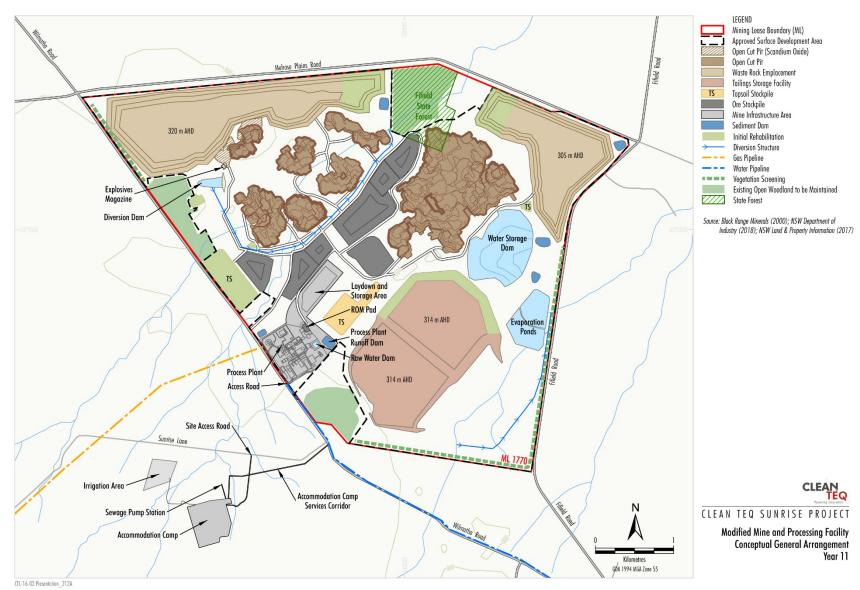
Figure 5: Mine and Processing Facility – Year 11
