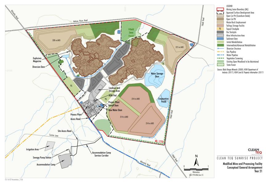
Figure 6: Mine and Processing Facility – Year 21
