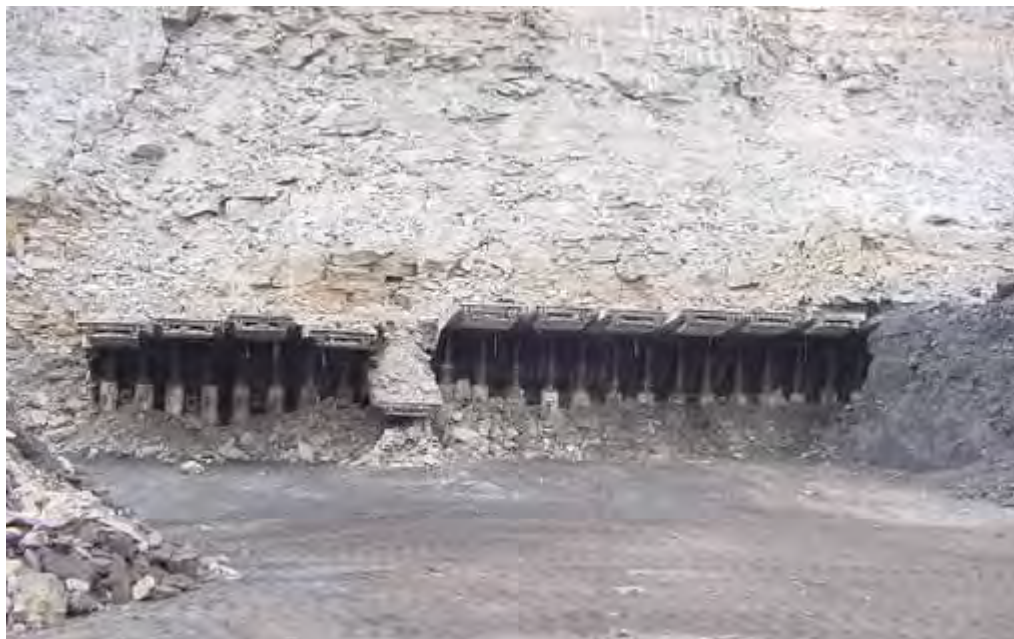
Figure I1. Photograph of a fracture zone above a longwall
