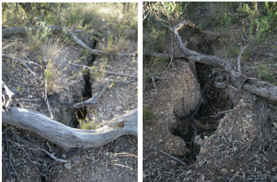
Fig. 4.4 Photographs of Surface Cracking at the NWUM
