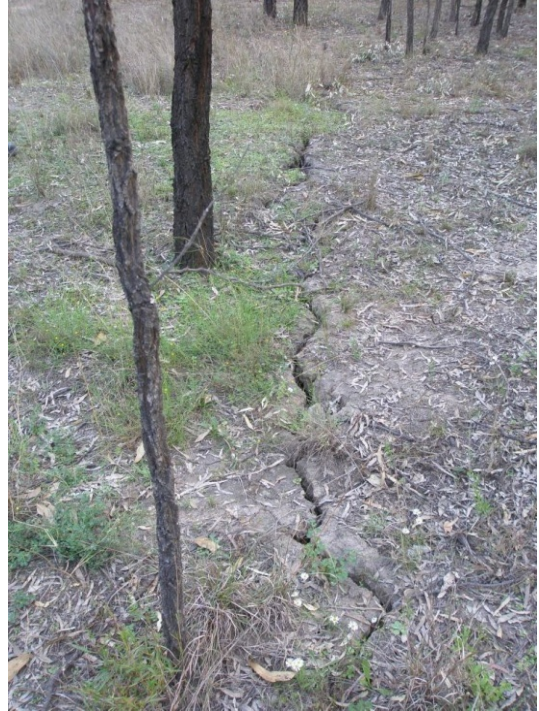
Plate 11. Typical soil cracking
