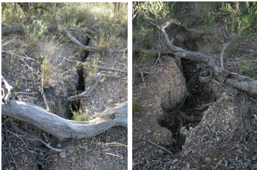
Fig. 4.4 Photographs of Surface Cracking at the NWUM
