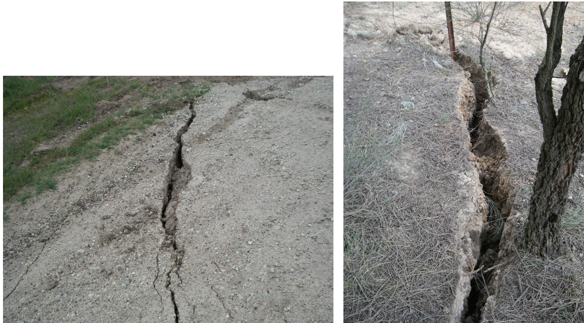
Fig. 4.5 Photographs of Surface Cracking above BSLW1 at the Blakefield South Mine
