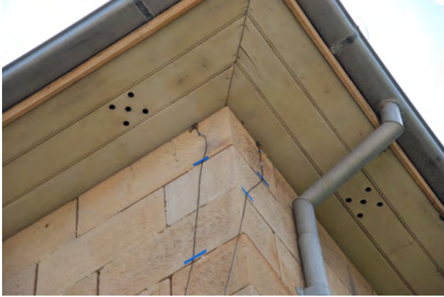
Figure 4: Accelerometers placed on the top south-western corner of Building 'A' to measure whole-of-building movement on two principal axes.
