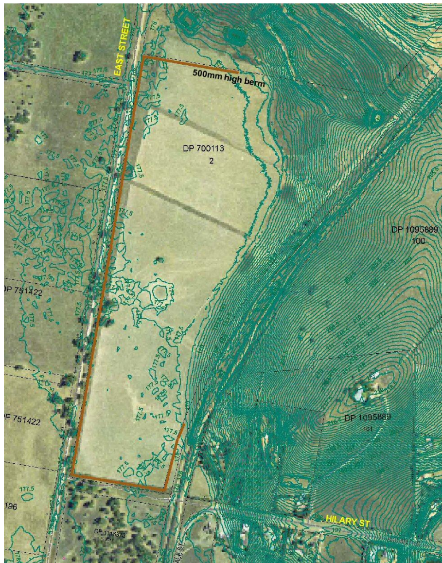
Figure 3 – Plan of CFA Low area showing location of low berm to protect downslope areas from natural runoff or excess irrigation water. The plan shows the 0.5 metre contours as provided by Wagga Wagga Council. All the 0.5 m contours on the irrigation area are either 177.0m contours or 177.5m contours giving an indication of how flat the site is. There is no major slope.
