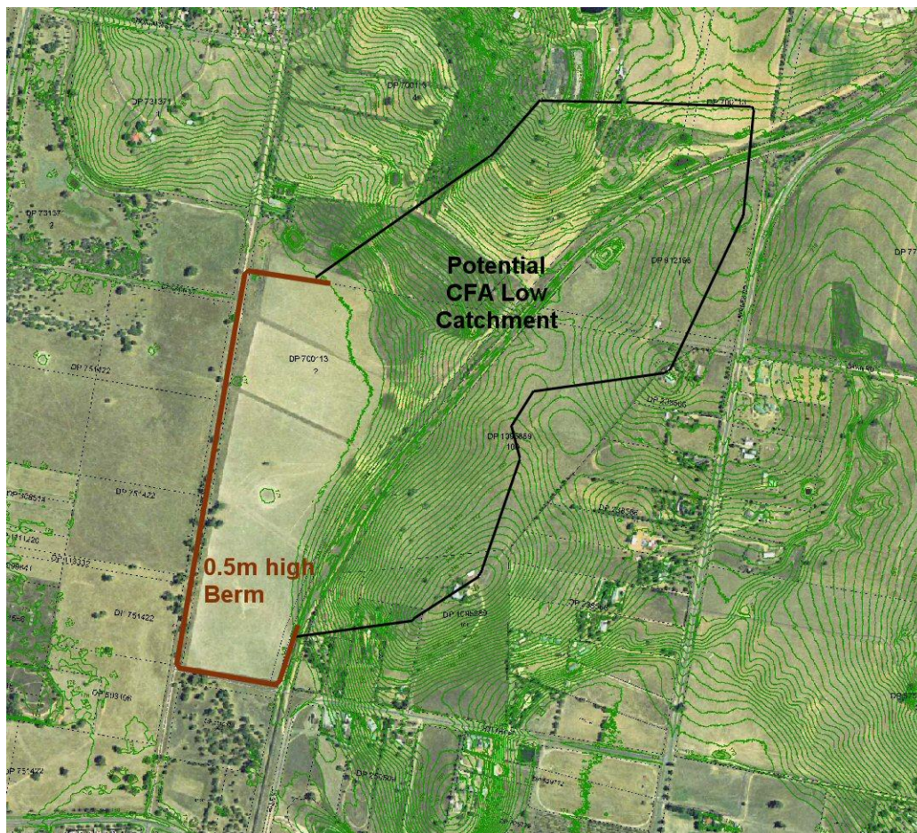
Figure 5 – 1.0 metre contour drawing from Wagga Wagga City Council modified to show the 0.5m berm and the Potential Catchment that may flow to the CFA Low irrigation area. The Potential CFA Low catchment is also shown estimated at about 100 hectares total.
