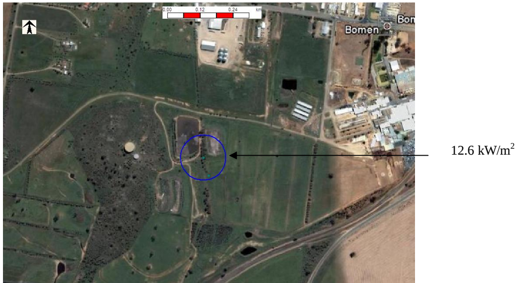
Figure 6-3 Thermal Radiation from a Fireball – 12.6kW/m 2
