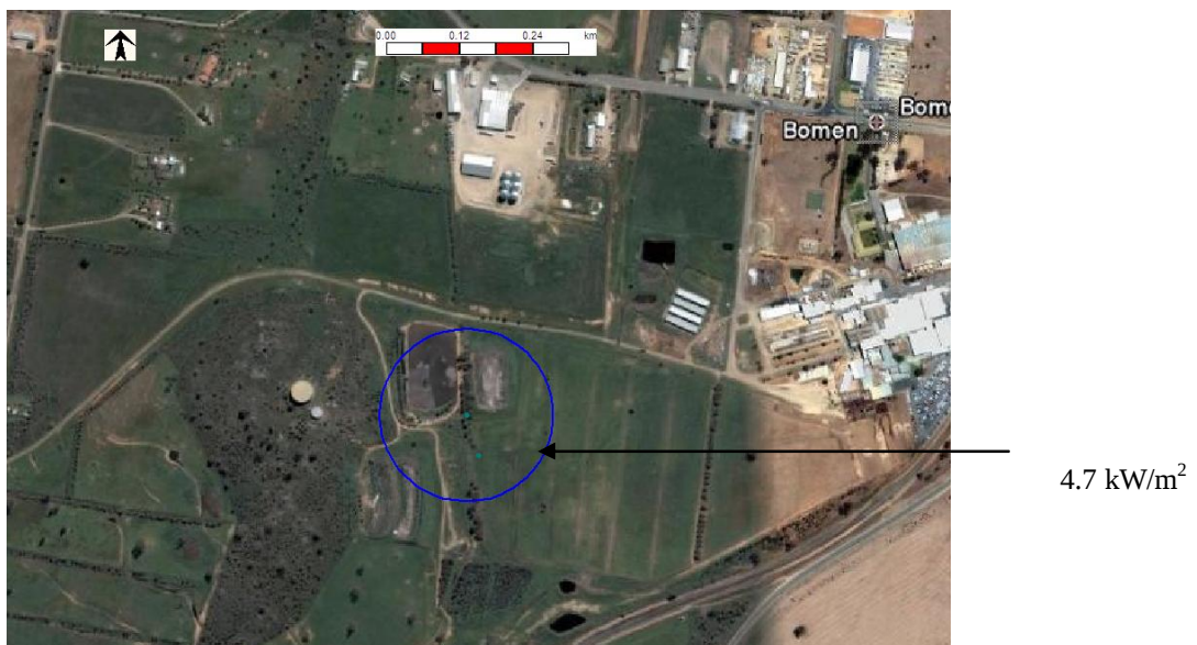
Figure 6-4 Thermal Radiation from a Fireball – 4.7kW/m 2
