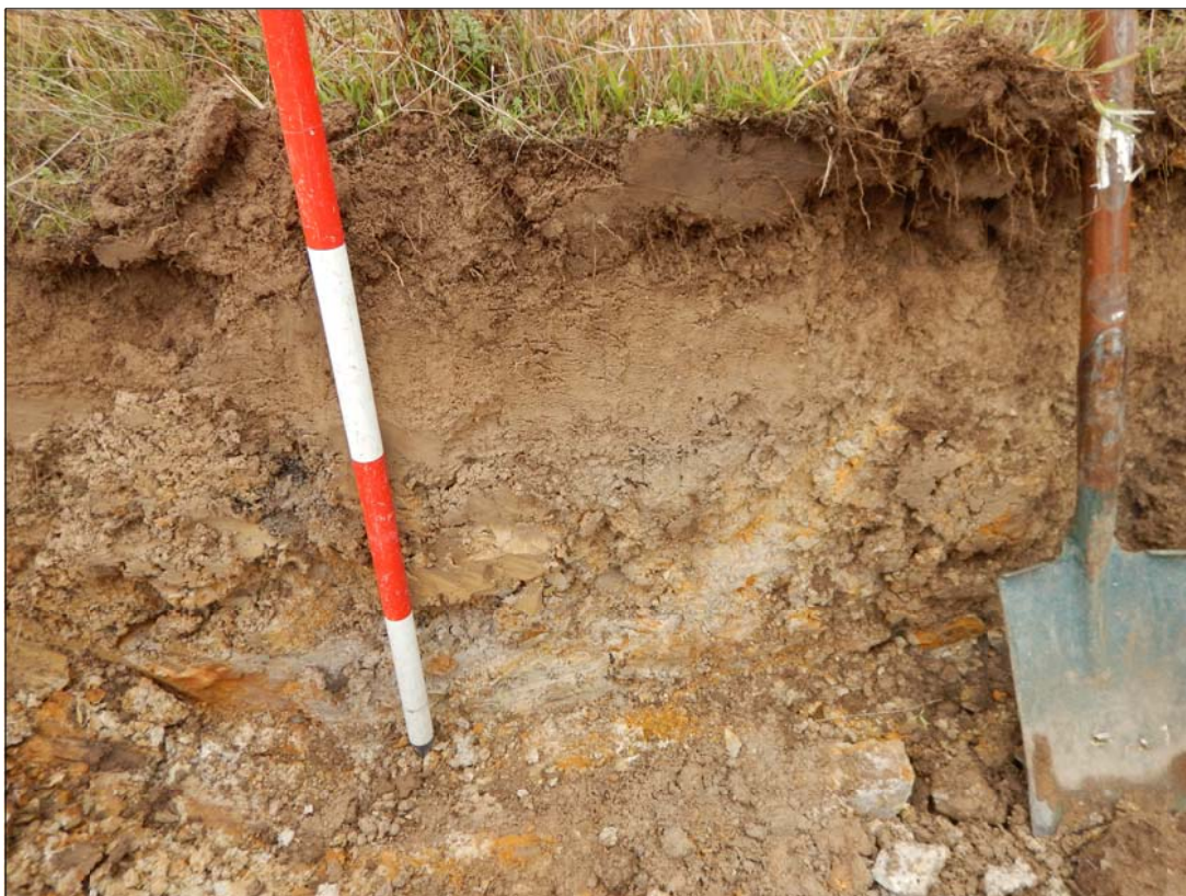
PLATE 4.2 Profile form at Site 28. Weathering mudstone is expose below 67cm in the profile
