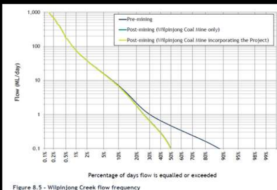
Figure 37. Flow exceedance curve for modelled flows in Wilpinjong Creek (left) and modelled flows for Wilpinjong Creek at Cumbo Creek (right). Sources: WRM 2015 (left) and WRM 2025 (right).
